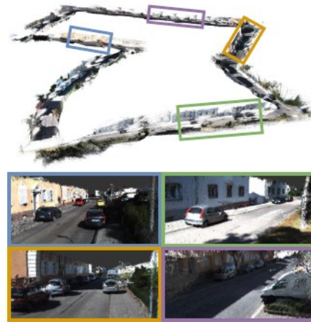
Figure 1: MonoRec can deliver high-quality dense reconstruction from a single moving camera. The figure shows an example of a large-scale outdoor point cloud reconstruction (KITTI Odometry sequence 07) by simply accumulating predicted depth maps. Please refer to our project page for the video of the entire reconstruction of the sequence.
